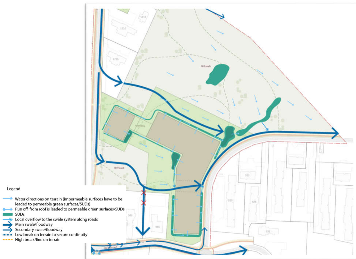
Figure 11: Detailed stormwater plan for school plot and public park.
